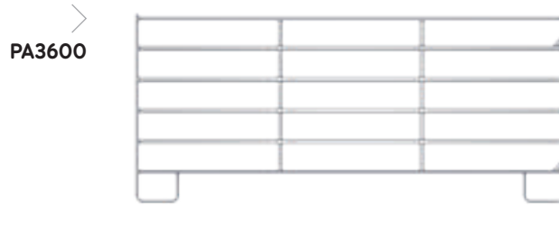
PA3600 Panel 3.60 m - With 2 vertical reinforcements - Available in packs of 16
